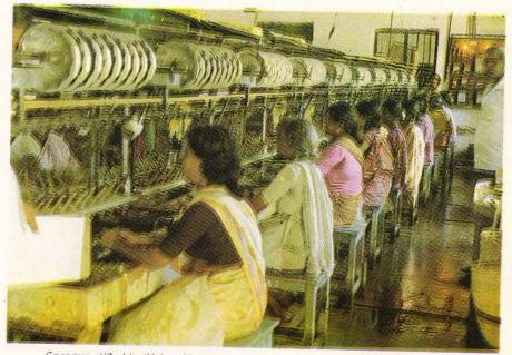
Cocoons stifled in 'Ushna Kothi' were reeled on cottage basin for large scale reeling trials. It was observed that reeling performances of hot air stifled cocoons in 'Ushna Kothi' is at par with that of steam stifled cocoons.
