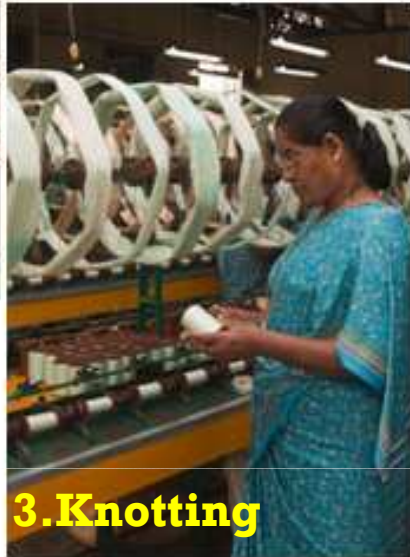
4. Winding under progress on to double flanged bobbins which rotates by surface contact
