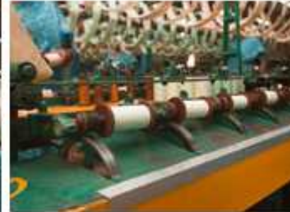
4. Winding under progress on to double flanged bobbins which rotates by surface contact
