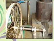
Sri Shivaiah owns a reeling unit at his native, Honnur. He had been experiencing power failure which indeed has obstructed his reeling work. To overcome this problem, he devised a hand pump by using a pulley and connecting it to the wheel of a bicycle using a rope. When the cycle is pedaled, the motor works and water is pumped to the boiler. It costs Rs.400/- and already eleven reelers have adopted this technology.
