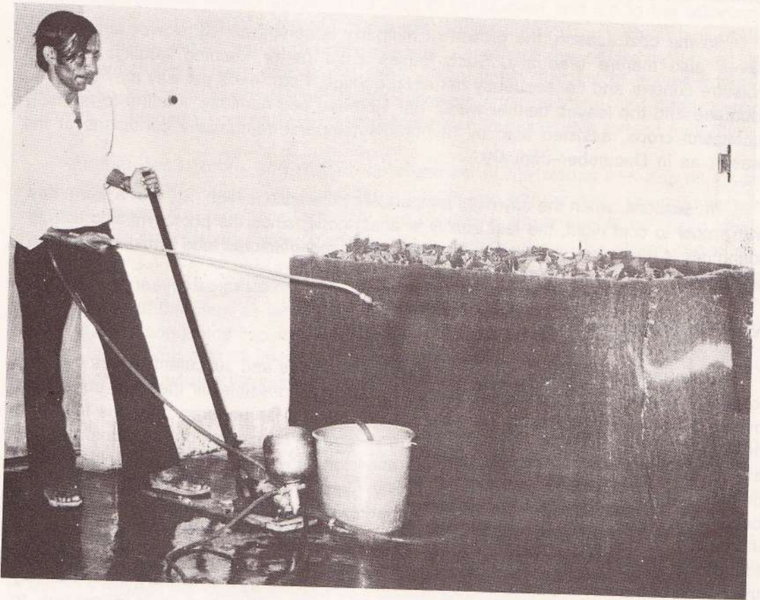
Figure 1 — Leaf storage bin being sprayed with water repeatedly during summer months
