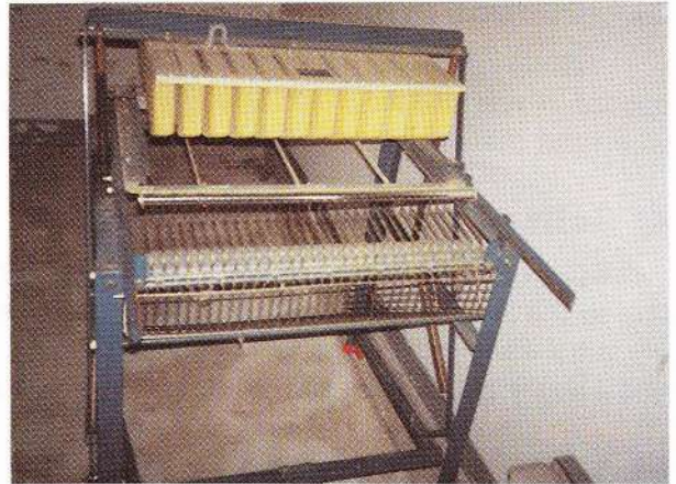
Fig. 10. Cocoon harvester for rotary moutage
