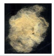
Cookers Waste: This grade produced during cocoon cooking followed by brushing, constitutes outer most layer i.e., floss. This grade has more sericin when compared to other grade wastes. It is rough in nature and hard to feel. It is 2<sup>nd</sup> grade waste.
