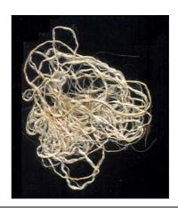
Reelers Waste: It is produced during reeling i.e., while feeding the ends, knotting of threads etc.,. It is not hard as in case of cookers waste. It is considered as 1<sup>st</sup> grade waste. Sericin content is less when compared to other grades. Also, the wastes produced during the process of silk throwing comes under this grade.
