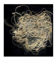
**Basin Waste/Refusal:** It is a waste left out in the bottom of the reeling basin while reeling. It constitutes palade layer. It is 3<sup>rd</sup> grade waste. The sericin content is very less and filaments are very thin.
