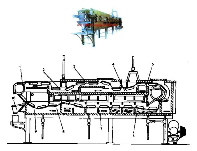
1.Cocoon hopper part, 2. Soaking part, 3.High temperature permeating part, 4.low temperature permeating part, 5. Cooking part, 6-7.Adjusting part, 8-9.Low temperature finishing part, 10. Cocoon outlet.
