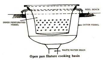
This method of cooking though simple is technically defective. The outer layers of the cocoon in contact with hot water get cooked earlier than the middle or inner layers and if the cooking is continued till these layers also get properly cooked, the outer layer gets overcooked. This results in unnecessary dissolution or over-softening of the gum which causes the filament to come off in lump and also spoils the cohesion, lustre and cleanness of the reeled silk.
